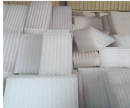
Inclined Tube Settler
